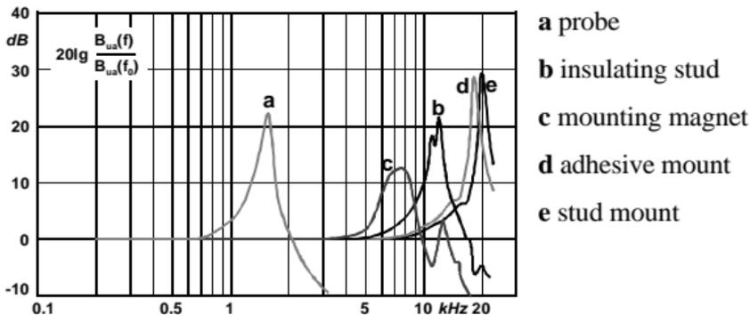
Figure 9: Resonance frequencies of different mounting methods
