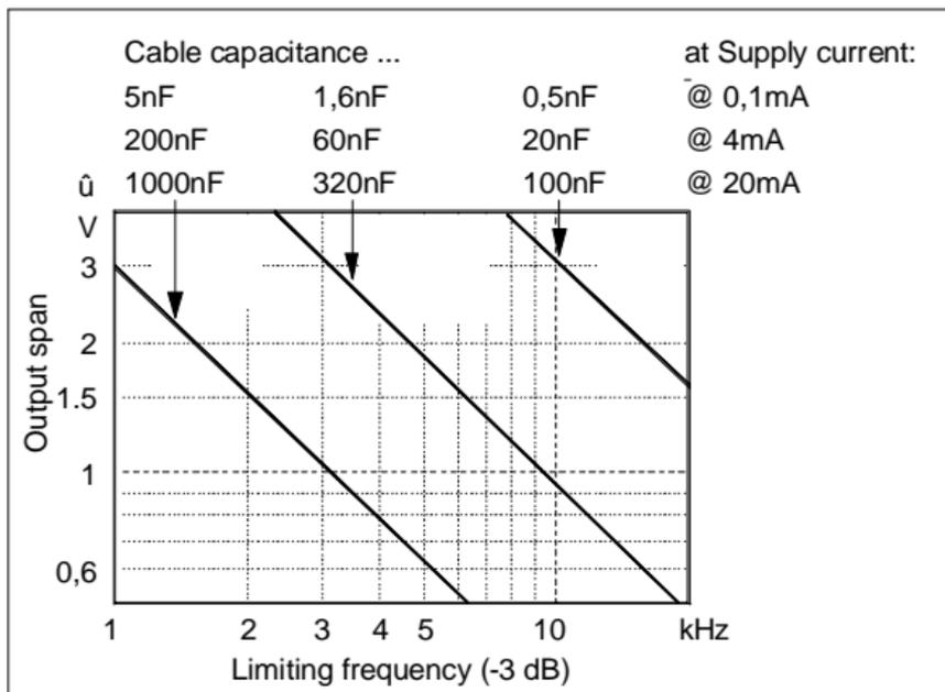
Figure 8 Output span of integrated preamplifiers
