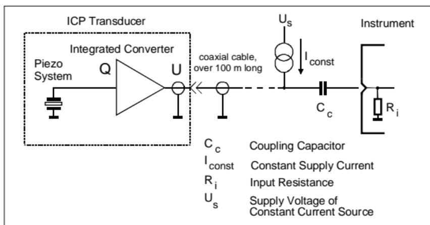
Figure 6: ICP<sup>®</sup> principle
