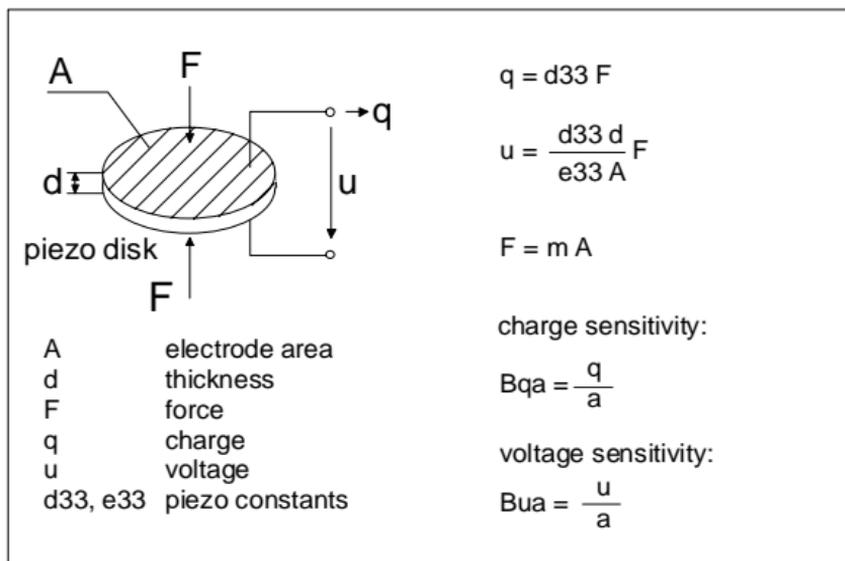
Figure 1: Piezoelectric effect, basic calculations
