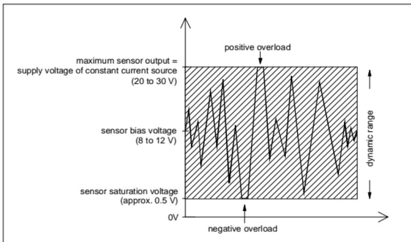
Figure 7: Dynamic range of ICP<sup>®</sup> compatible transducers
